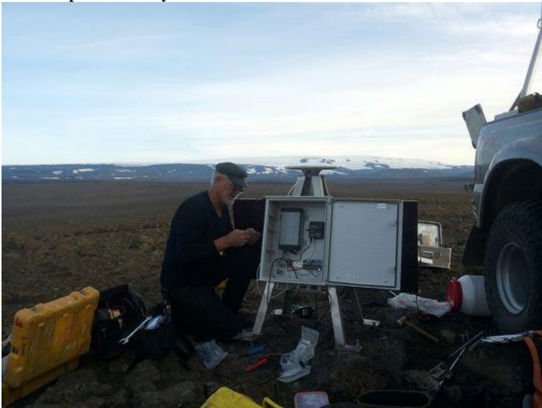
A new GPS station being mounted near Gjallandi, north of Vonarskarð. Bárðarbunga in the distance. Þorsteinn Jónsson working. Photo: Benedikt G. Ófeigsson.
